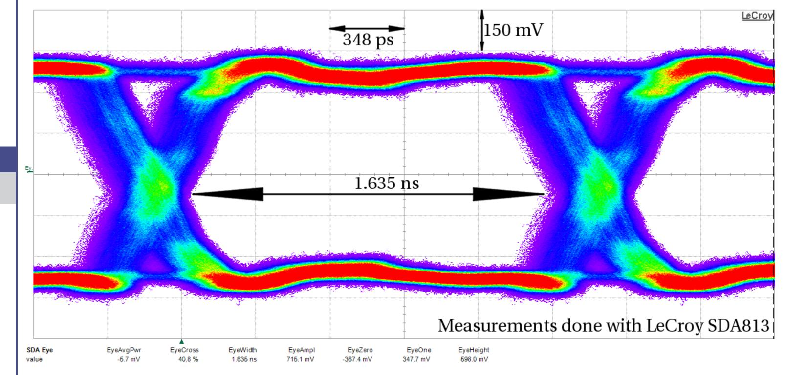
Implemented using DDR I/O. 3 serialisers occupy <2% of the XC3S400A + 1 DCM
