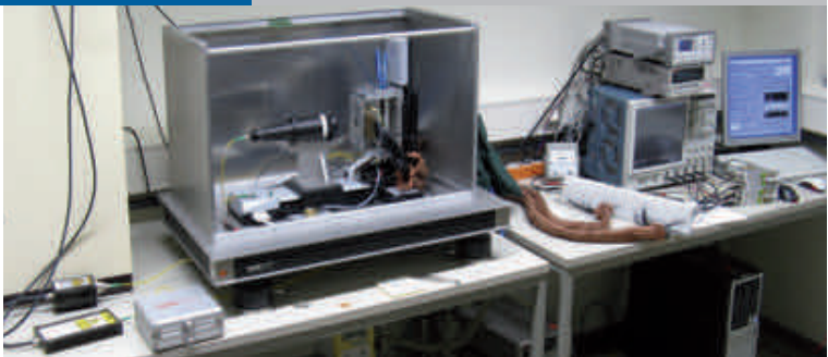
Figure 2: The multi-channel TCT set-up in Hamburg.
